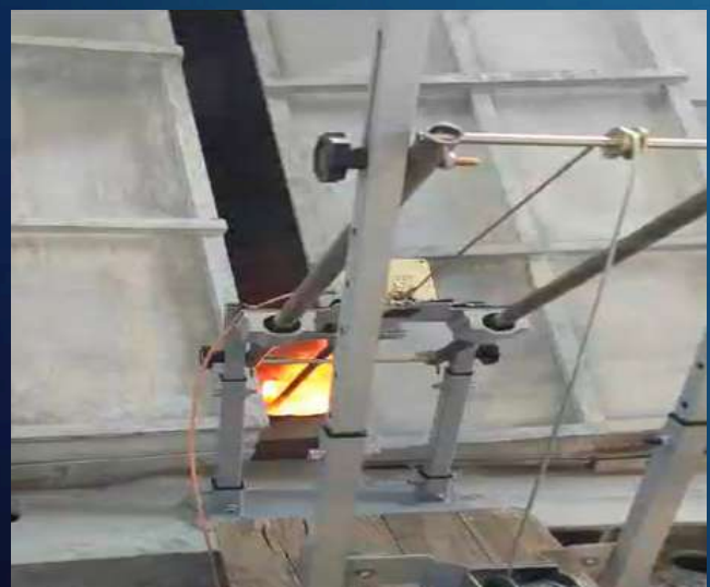
Ultrasonic Waveguide for Molten Metals Cryolite Bath and Measurements up to 1400 ^{\circ}\text{C}
