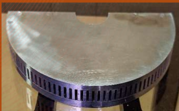
Cylindrical hyperlens fabricated at CNDE for Far-field Imaging
