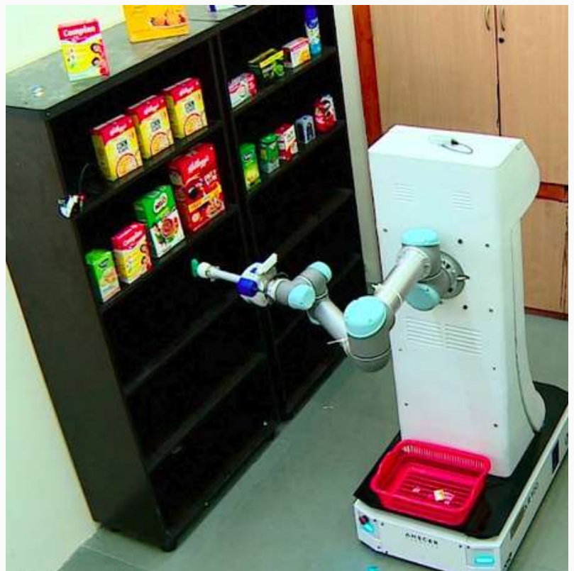
Pictures of the Shobot in the arena while picking the carton box from the shelf
